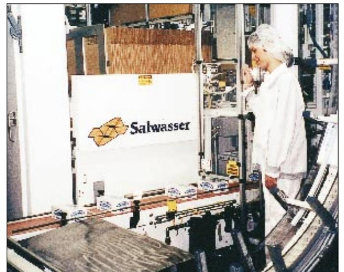
A primary feature of each packer is a specially-designed loading tube that actually protects the rather lightweight cartons as they are lifted and loaded into the corrugated cases. The tube essentially eliminates any potential crushing that occurs when the cartons’ corners or edges catch on the case edges and corners during the load cycle.
