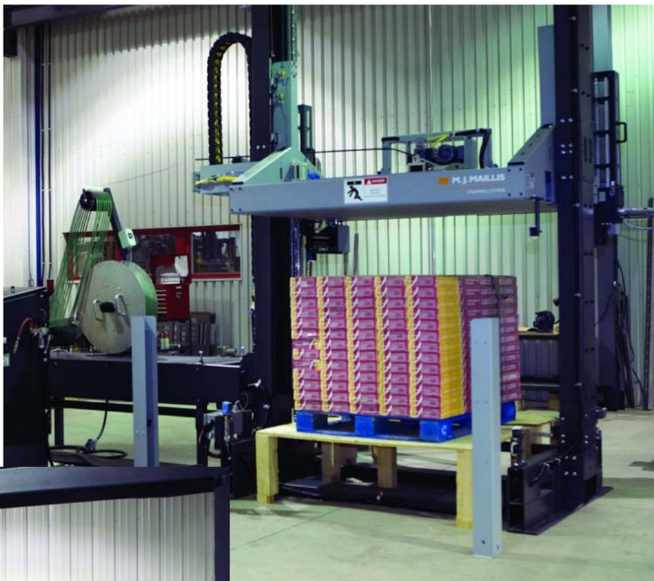
Thanks to the melding of companies, Wulftec now manufactures M.J. Maillis strapping machines, like this fully-automatic Vario Master 9461 machine with compression force up to 2,200 pounds.
