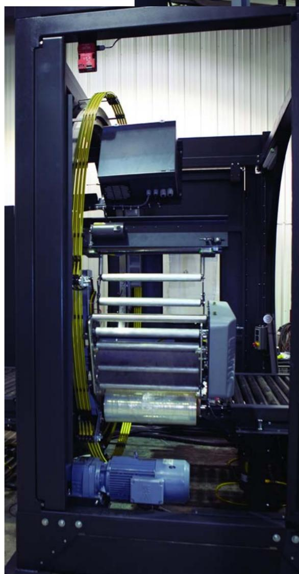
A SEW Eurodrive motor powers the film carriage of the WRVA-200 automatic horizontal stretchwraper.
