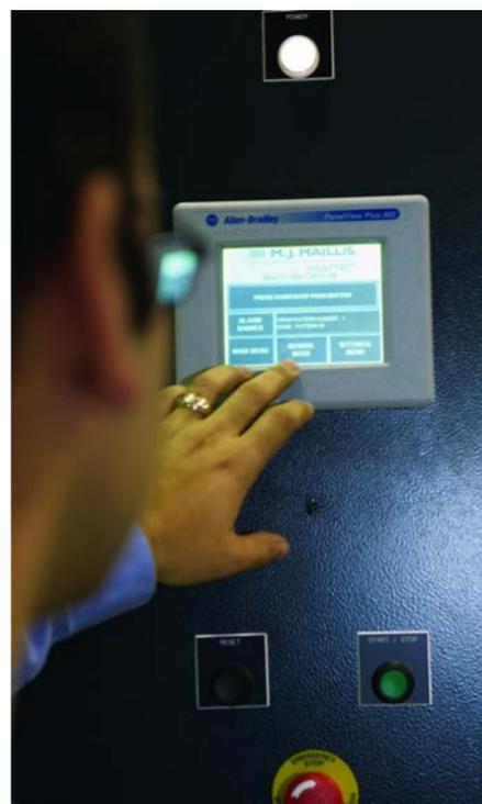
Yanick Marois uses an Allen-Bradley touchscreen interface to program functions onto a WCRT-200 rotary-arm, fully-automatic stretchwrapper.
