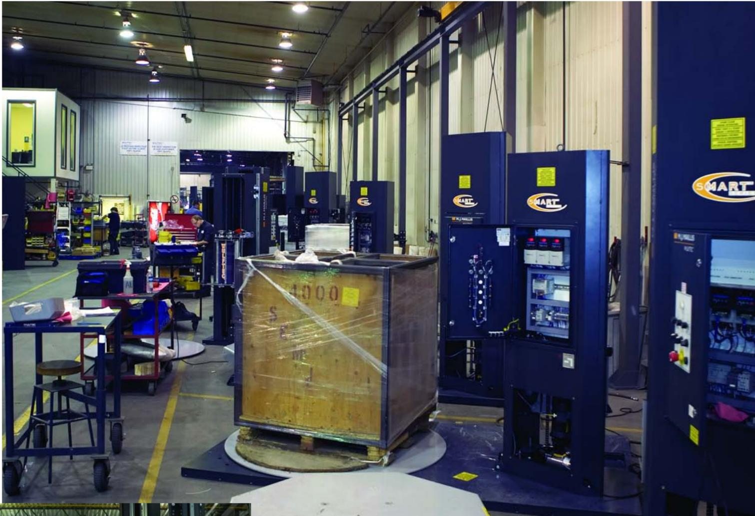
A production line dedicated to manufacturing of modular, semi-automatic Smart Series stretchwrappers.
