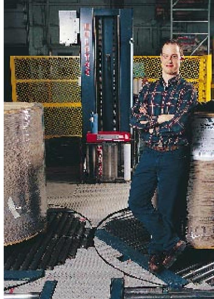
Cascades Conversion plant engineer Martin Caya poses with the company's Wulftec WCA-200 dual-turnstile stretchwrapper. The two turntables help keep Cascades' packaging operation moving efficiently.
