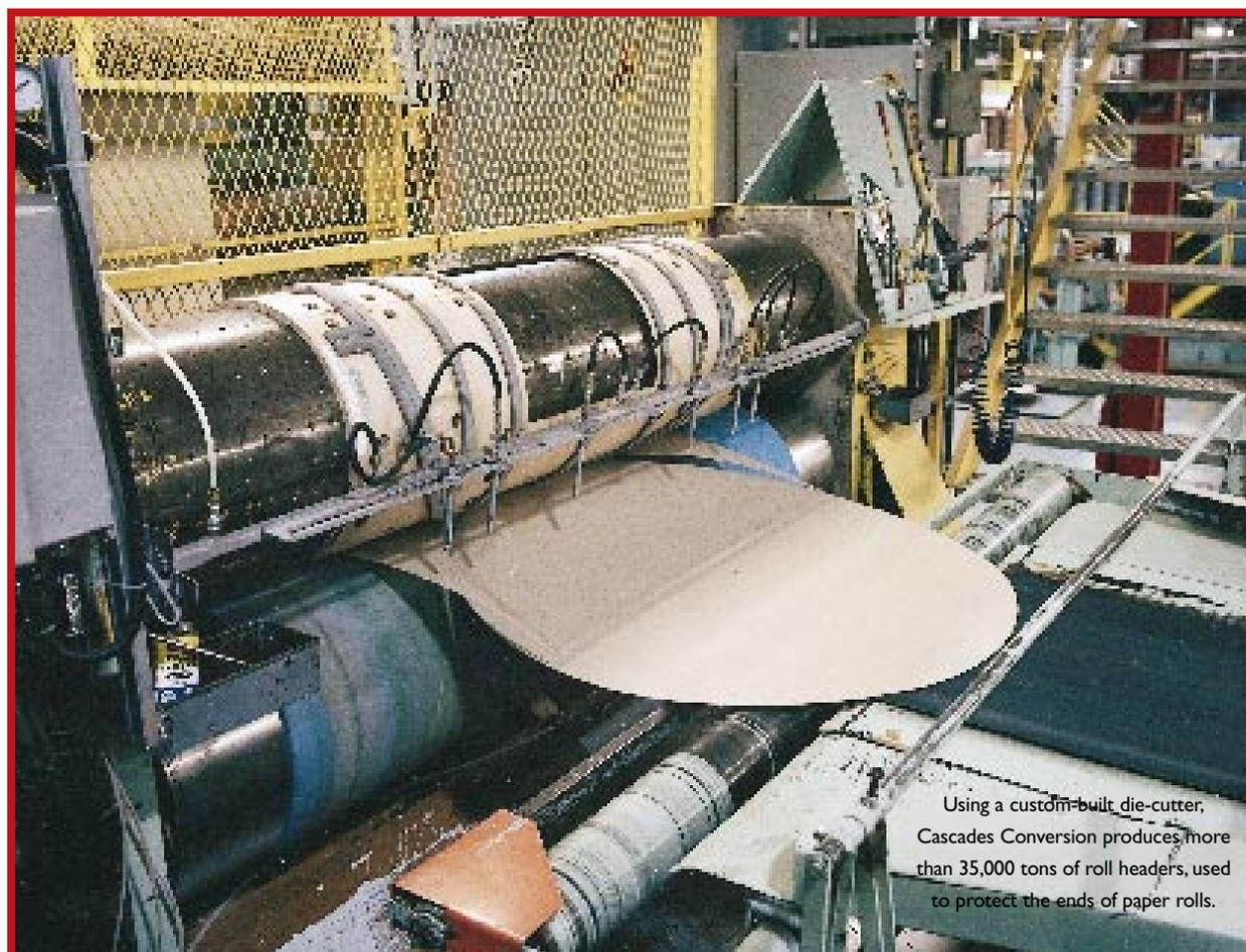
Using a custom-built die-cutter, Cascades Conversion produces more than 35,000 tons of roll headers, used to protect the ends of paper rolls.
