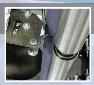
Save precious time by adding a Rapid-Cut device to puncture the film at the end of the cycle to separate the film from the load. For a very small upcharge, increase you throughput on your semiautomatic stretch wrapper and reduce film usage by shortening the film tail versus the usual operation of cutting with a knife. With this method, you can easily position the tear at a corner of the load. The Rapid-Cut can easily be retrofitted on existing equipment.
